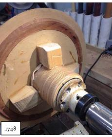
cobs chuck and 1 1/4 inch Forstner bit, the pilot hole is bored. The tap is then mounted in the tailstock with a four-jaw chuck (because the tap has a four-sided shank, a Jacobs chuck will not work). With the headstock locked, the tap is slowly rotated and fed into the pilot hole. Unlike thread chasing, the lathe is not turned on. Even if your lathe could run in the
